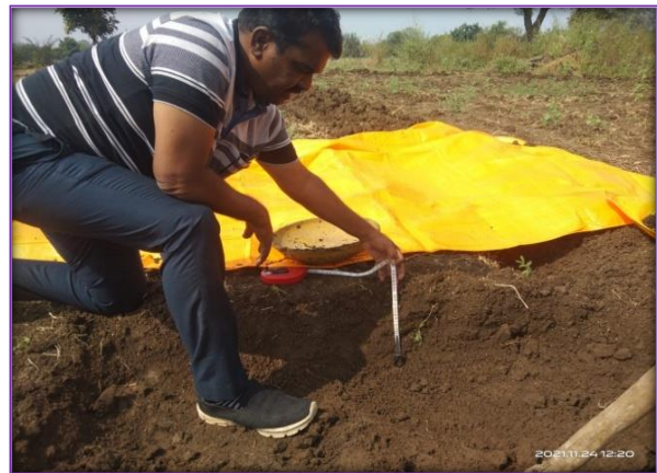
Plate 2: Manual excavation of pits and measurement of the depth
